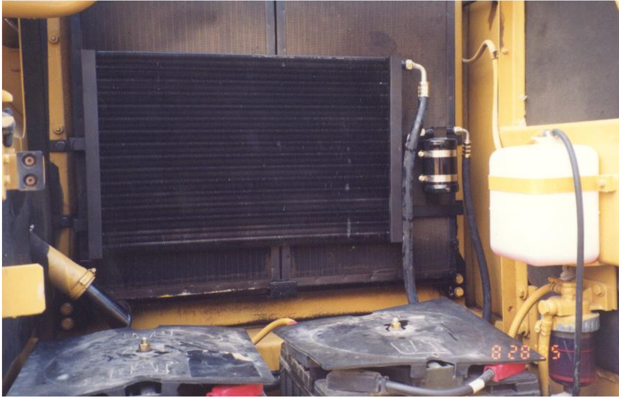
Condenser in place with attached drier and hoses (322L).
