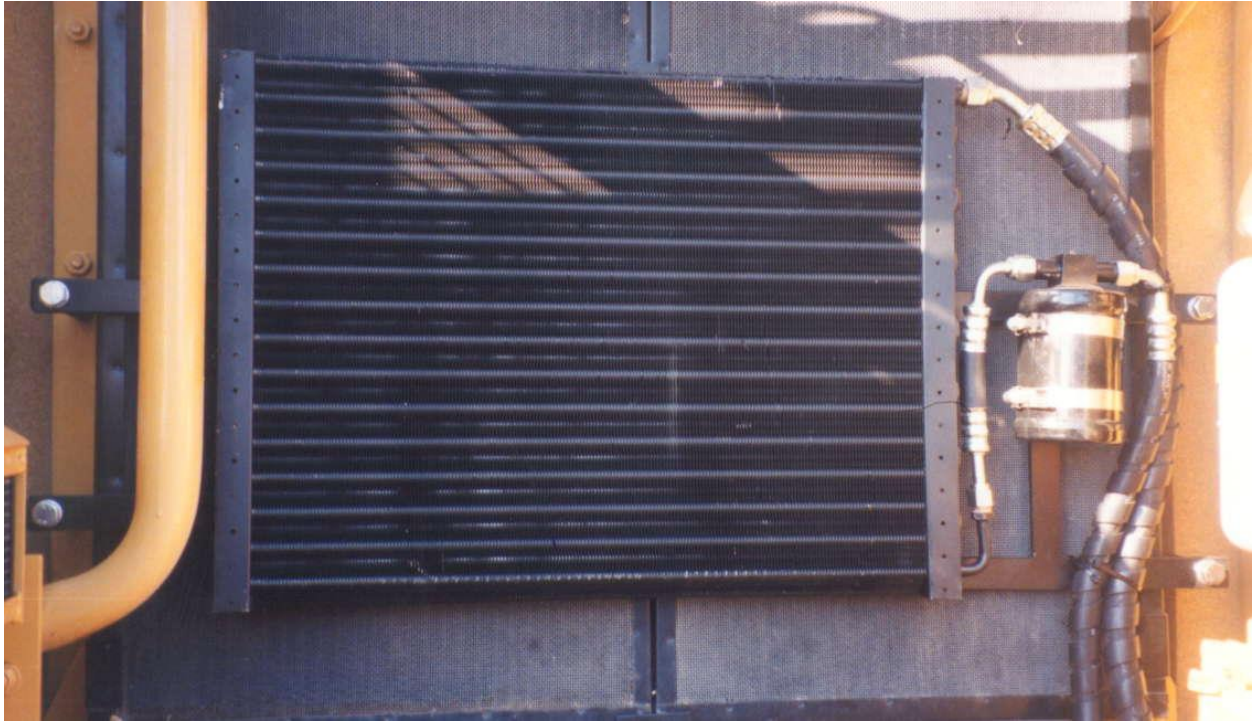
Condenser in place on 322B series excavator.
